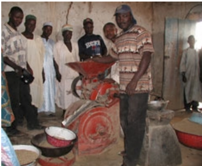
Small-scale paddy dehullers provide the bulk of processing capacity in Nigeria
